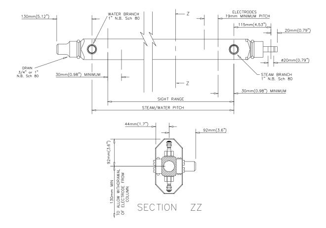
Figure 1.2 - Low pressure water column (120bar, 1740psi)
